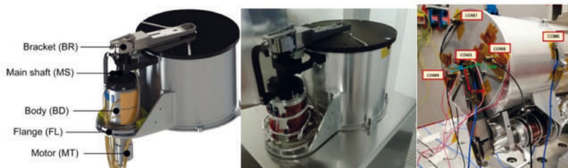
COM subsystem and its components in rendering (left), flight model (centre), during vibration tests (right).
