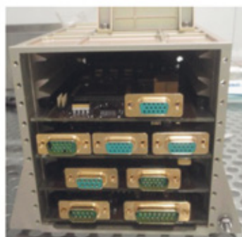
Example of Modularity of CEU configuration using different board configuration on common backbone
