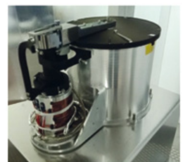
[3] Janus' Front Door mechanism and its subsystems (above); the JANUS COM FM during testing (right)
