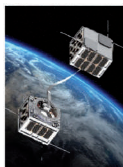
Fig. 1. E.T. PACK 12U demo flight with the Electron Emitter Module (EEM) and the Deployment Mechanism Module (DMM) connected by a tape tether.
