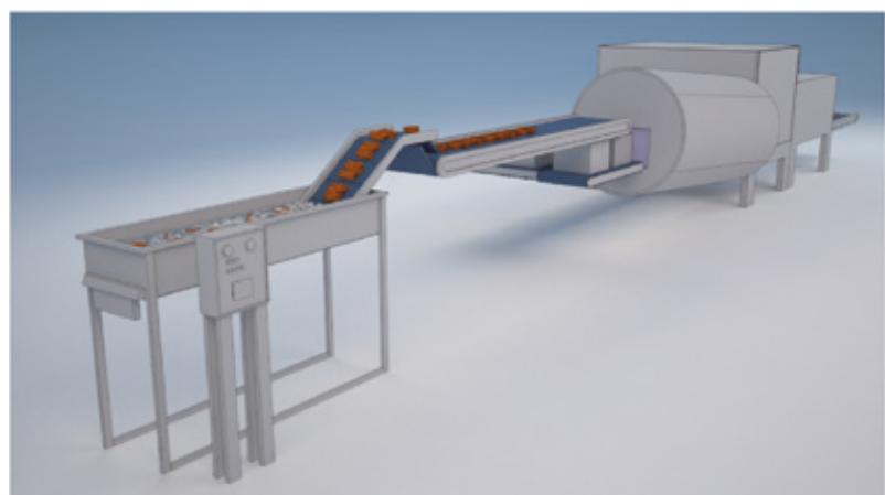
High pressure CO<sub>2</sub> pasteurization continuous plant for solid products
