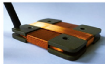
Figure1: new three-axes pick-up sensor (left) and system layout (right) of the RFXmod2 experiment
